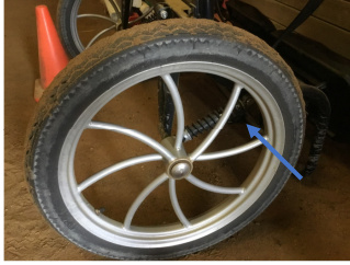
Pneumatic tire and spiral spring
